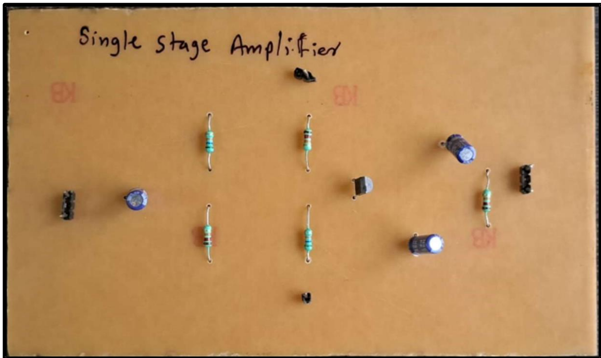
Figure: Circuit implementation on PCB (Single Stage Amplifier)
