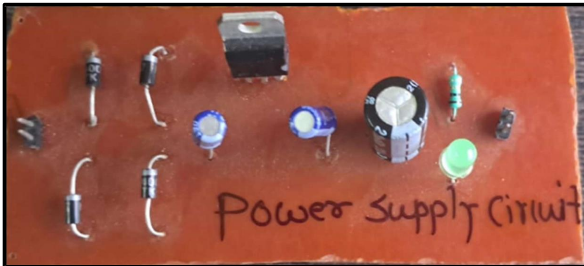
Figure: Circuit implementation on PCB (Power Supply)
